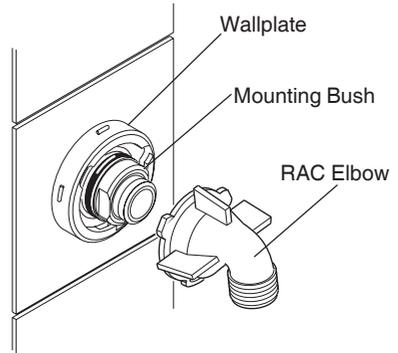
**2.10.** Rotate the RAC elbow clockwise to lock it in position. A 'click' will confirm that the RAC elbow is locked.
