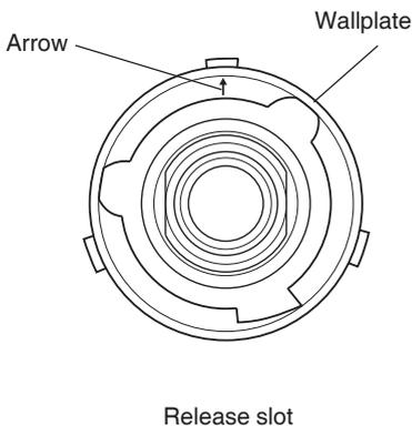
**2.7.** Rotate the wallplate to align the elbow release slot at bottom centre, and with the arrow pointing upwards.
