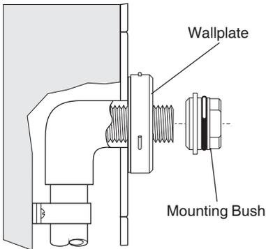
**2.6.** Screw the mounting bush on to the brass nipple until it clamps the wallplate loosely against the wall.
