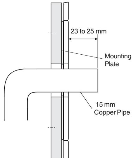
**4.12.** Fix the backplate to the wall using the two fixing screws.
