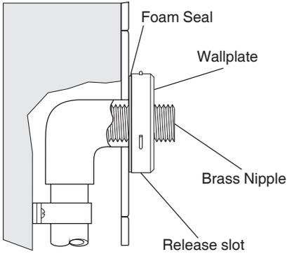
**2.4.** Place the wallplate over the brass nipple. Make sure that the foam seal abuts the finished wall surface.
