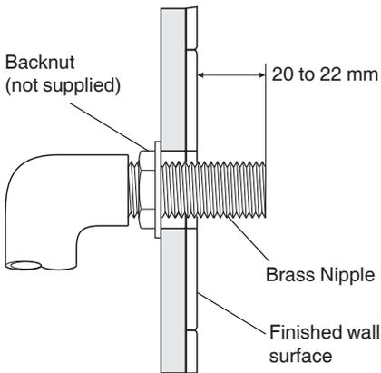
**3.1.** The supply pipe from the shower control must terminate with a 1/2" BSP female thread.
