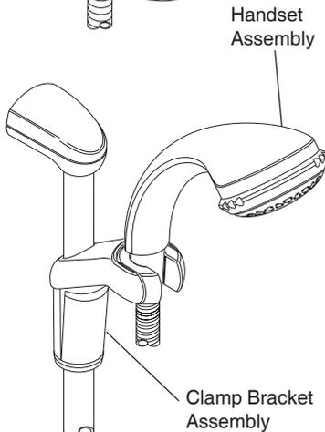
**1.13.** Place the handset assembly in the clamp bracket assembly.
