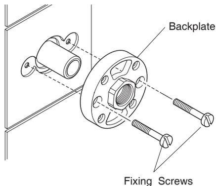
**4.13.** Fit the compression olive over the copper pipe and tighten the backplate nut into position. Flats are provided on the wallplate and backplate nut for a 24 mm A/F spanner.
