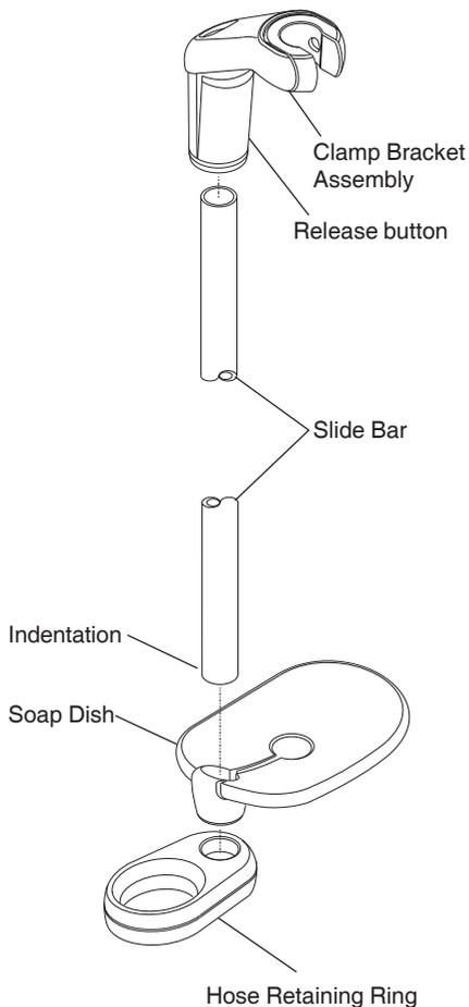
**1.3.** Depress the release button on the clamp bracket assembly and slide the clamp bracket assembly on to the slide bar. The slide bar has an indentation at one end that should engage in the lower slide bar support body.
