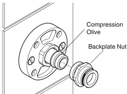
**4.14.** Ensure the 'O' seal is fitted on the backplate nut. Push the bir assembly over the backplate nut onto the wallplate.
