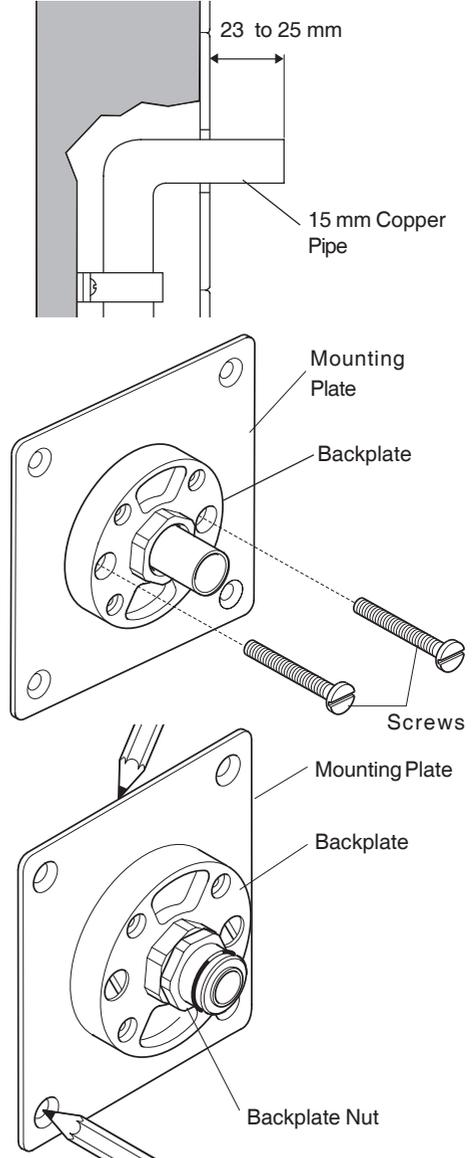
**4.7.** Drill the four mounting plate fixing holes. If necessary, make a recess approximately 6 mm deep to accept the mounting plate. Fit the four wall plugs supplied to the fixing holes.
