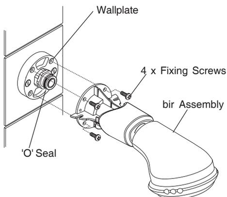
**4.16.** Fix the upper shroud to the bir assembly using the four self-tapping screws provided.
