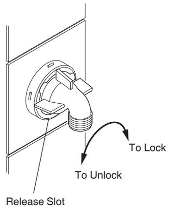
**2.11.** Locate the RAC shroud over the RAC elbow. Carefully push the shroud until it engages with the lugs on the wallplate.
