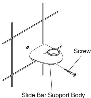
**1.6.** Use the screw provided to fix the bottom slide bar support body to the wall. Do not fully tighten the screw to make aligning the top slide bar support body easier.
