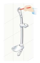
Mark the position of the middle slot on both top and bottom Supports.
