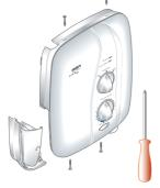
Refit the Service Tunnel and Cover. Make sure they fit correctly.
