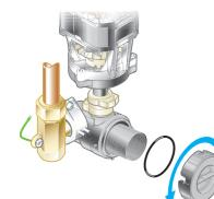
Press down on the filter cover and turn anti-clockwise to release.
