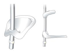
Slide the Soap Dish/Hose Retaining Ring and the Soap Dish Support collar onto the Slide Bar below the Clamp Bracket. 4.
